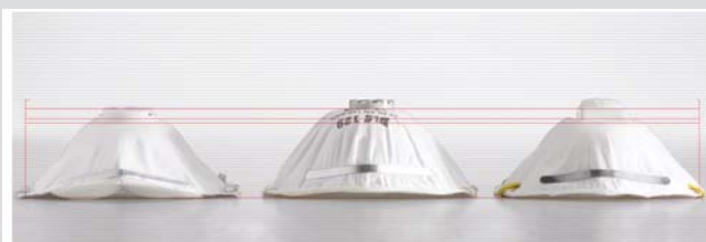
Filtering facepieces passed Dolomite dust clogging test. Lower breathing resistance, higher duration
